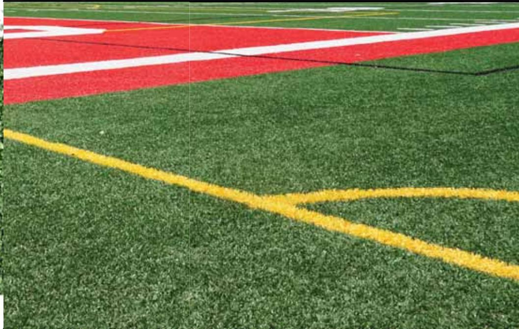
*SOF-TOUCH Performance Turf Granules provide a natural grass appearance, prevent premature turf wear, and offer excellent support for athletic field play. The high density of the EPDM granules also prevents migration during use and significantly reduces the elasticity or “bounce” associated with lower density materials, such as SBR rubber granules.*
